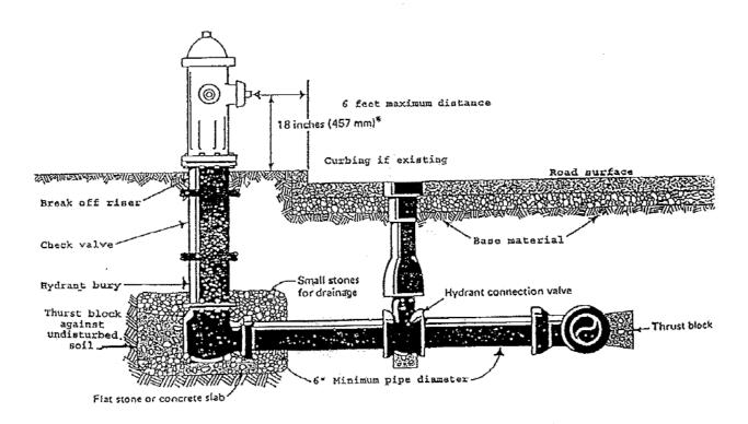
WHERE PAVED GUTTERS ARE INSTALLED THE CENTER OF THE HYDRANT SHALL BE NO MORE THAN 6 FEET FROM THE CENTER OF THE DIKE, INCLUDING SIDEWALKS.
